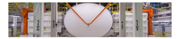
Jetskin® is a metallic coating for steel applied by JVD (Jet Vapor Deposition, where a coil is coated continuous in a vacuum chamber). This will allow a much lower ecological footprint. Jetskin® provides a homogeneous coating on one or both sides of the steel.
